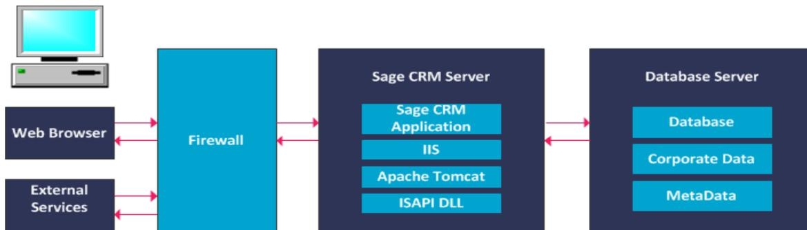
Sage CRM is a 32-bit application which can run on a 64-bit server. Sage CRM installations comprise of a Sage CRM server and a database server. As Sage CRM is a web-based solution, each user needs a web browser and IP connection to the Sage CRM server to access the system.
