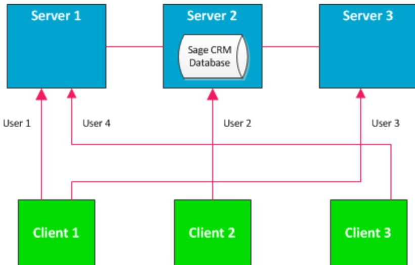
In this scenario, load balancing has been configured on a cluster of three servers: Server 1, Server 2, and Server 3. Each server can access the Sage CRM database which resides on Server 2. User 1 logs on from Client 1, then User 2 logs on from Client 2, then User 3 logs on from Client 1, and then User 4 logs on from Client 3.
